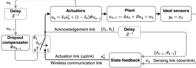
Fig. 1. Closed-loop system architecture. A wireless link delivers SF control inputs to actuators. The receiver measures the link state  $\theta_k$  and communicates it with the transmission outcome  $\delta_k$  to the controller. The actuators apply the generalized packet dropout compensation.
