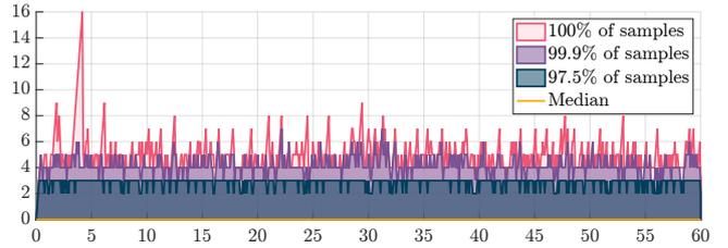
Fig. 7. Control-packet error burst length statistics over 60 seconds from a batch of 2000 traces: the median values (in orange) are all zero, 97.5% of observed values (in blue) are always less than or equal to two, 99.9% (in violet) is less than or equal to 7, and the maximal values (in red) are predominantly below 8, but equal 9 three times, and 16 once.
