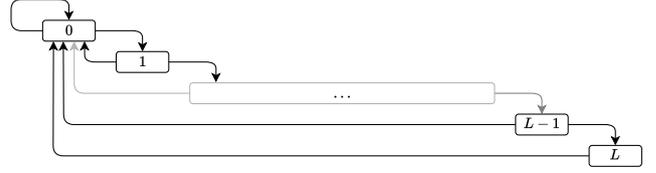
Fig. 4. Graphical representation of the stochastic process  $\{\Delta_{\tau(m+1)}\}$ : the rectangles mark the process states labeled with the values each random variable  $\Delta_{\tau(m+1)}$  can assume, and the directed arcs between states indicate the non-zero probability transitions from the current to the next state.
